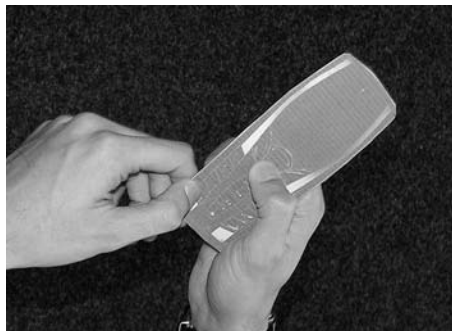
FIGURE 11.8 Simulating the size of a mobile phone in a child's hand.
