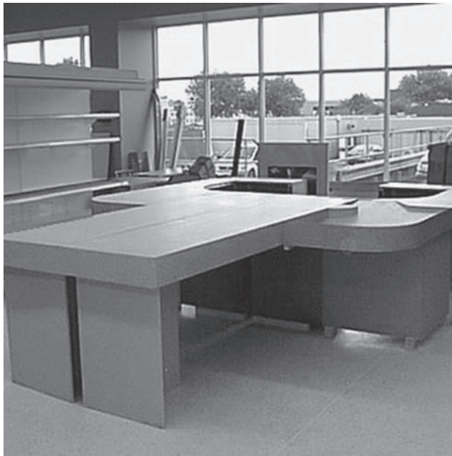
FIGURE 20.6 MDF mock-up of the “radical” checkout design.
