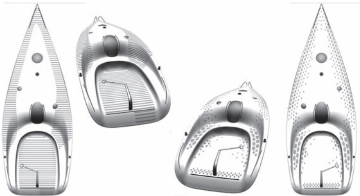
FIGURE 27.9 Two different macro-grip design solutions of deck surfaces according to guidelines.
