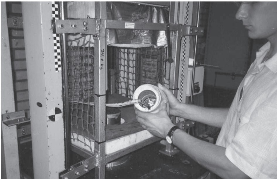
FIGURE 19.5 European helmet test rig. The helmet with the headform attached falls freely inside the steel cage.
