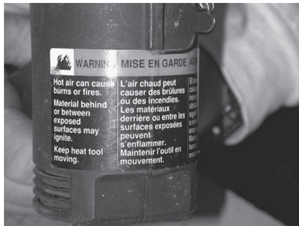
FIGURE 4.12 Warning on a heat gun.
